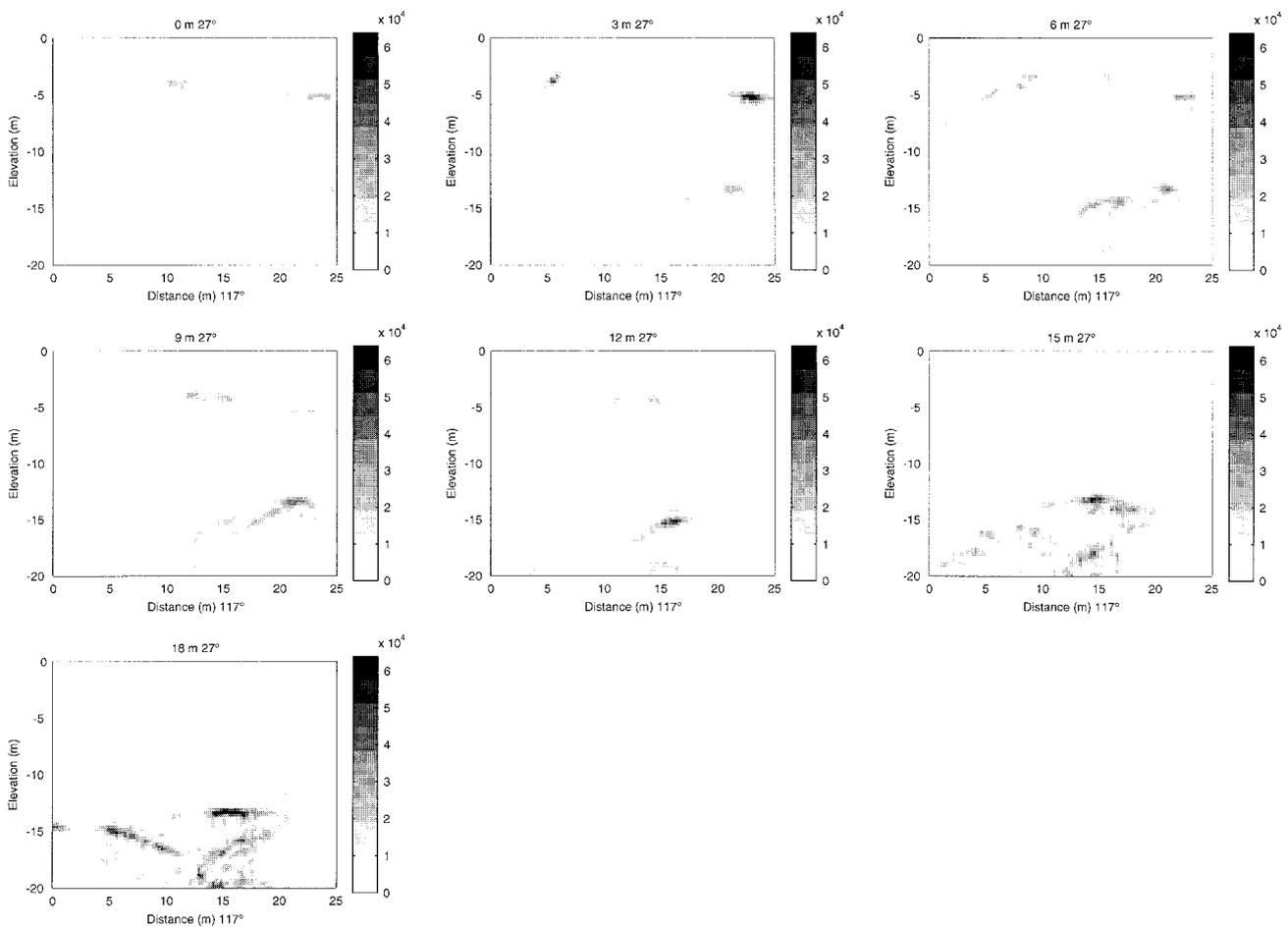
Figure 3. GPR data from parallel 25 m transects. Strength of reflection is measured on a ten-point grey-scale. Transects are oriented along the direction  $117^\circ$  from west (left) to east (right) and are separated by 3 m between adjacent transects. Note the prominent returns at 6 m and 14 m depths.
