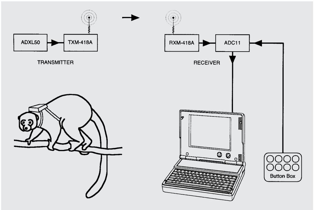
**Fig. 1.** Schematic diagram of the remote accelerometry equipment.
