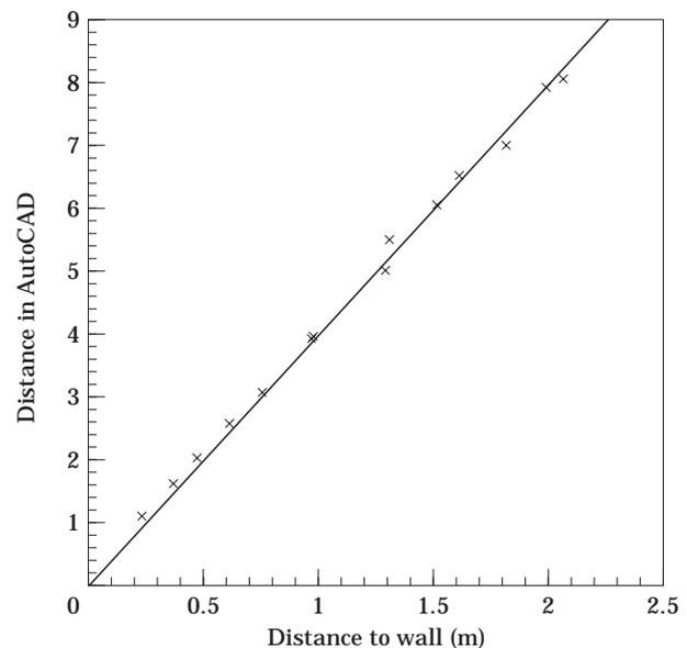
Figure 3. The relationship between scans of known distances and the distances in arbitrary AutoCAD units after tracing. The equation of the best fit straight line through the points is  $y=4.020x$  with  $r^2=0.9976$ . This relationship was then used to calibrate subsequent measurements.
